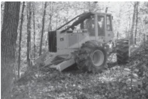
A skidder making a temporary water bar. Water bars used along with revegetation can help prevent roads and trails from eroding.
