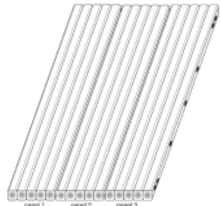
When constructed in the simplest form, the bridge panels are made from hardwood cants, fastened together with threaded rods. The panels are generally 4-6' wide, 8-10" thick and 16-32' long. The size you choose would depend on the width of the stream crossings you are likely to encounter, the size and type of your equipment and the load you need the bridge to support. In general the longer
